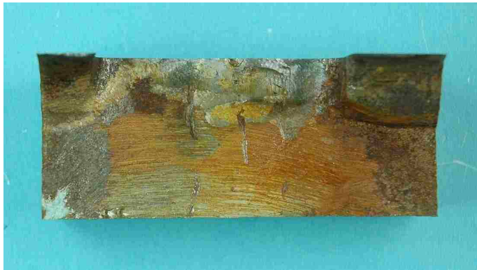
Figure 171 Weld root section 6 of CJP deck weld
