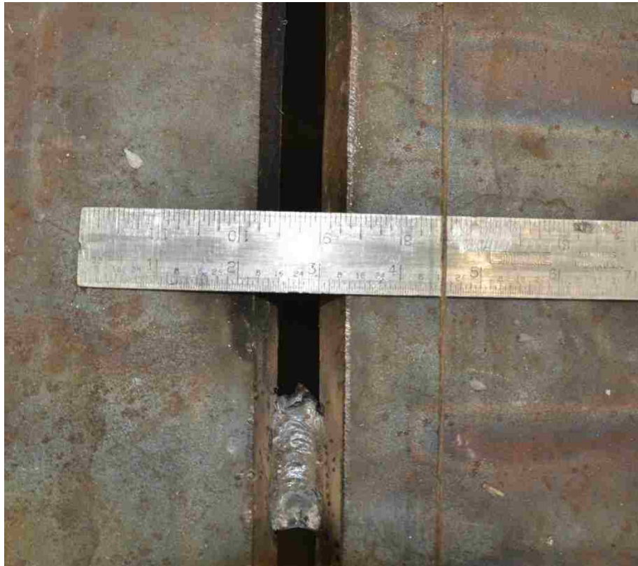
Figure 111 Maximum root gap of 1/2 in.
