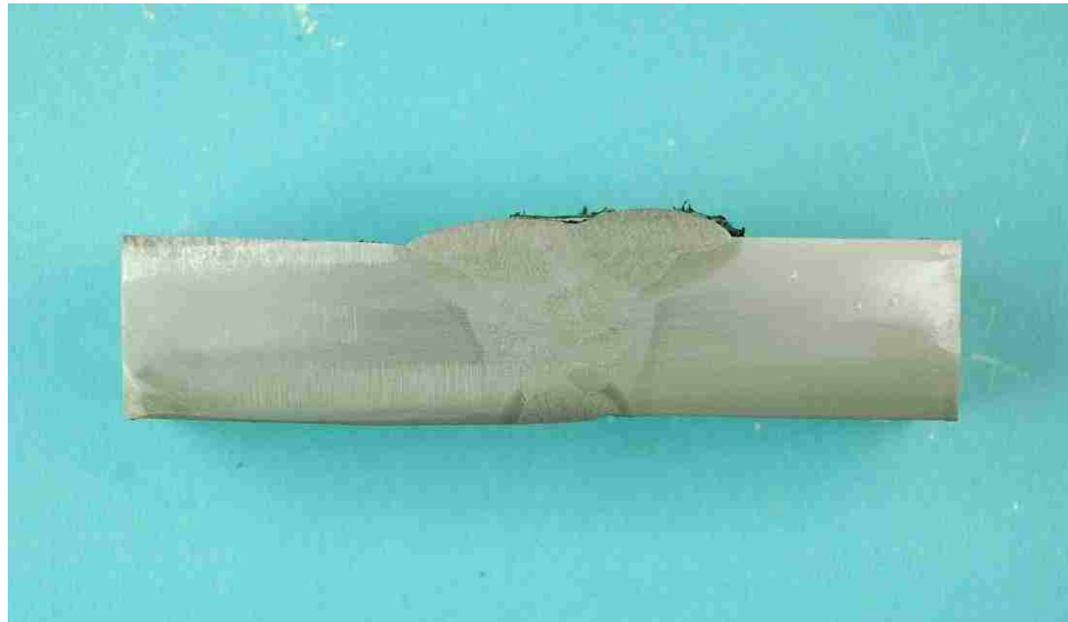
Figure 166 Macro-etched section 4 of CJP deck weld
