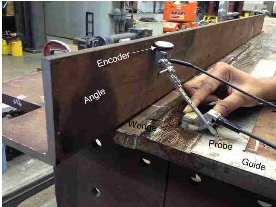
Figure 156 Scan setup in the laboratory
