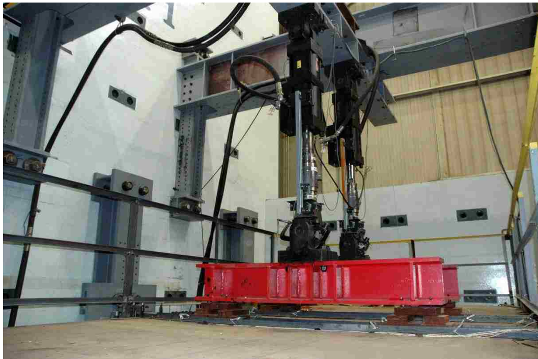
Figure 140 Arrangement of above-deck actuators
