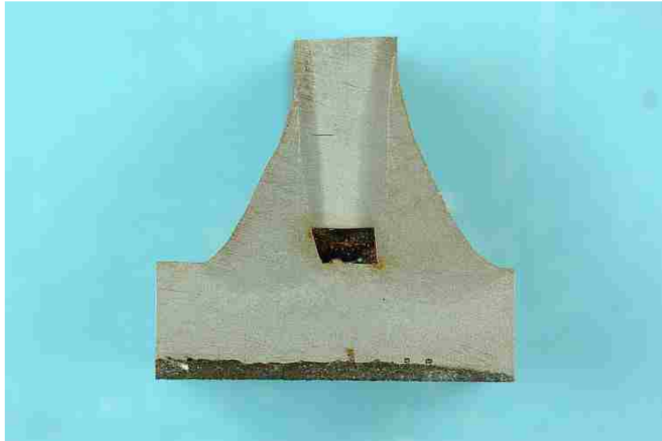
Figure 153 Macro-etched section FS_S_C
