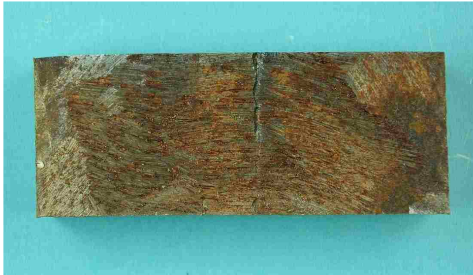
Figure 174 Weld root section 7 of CJP deck weld
