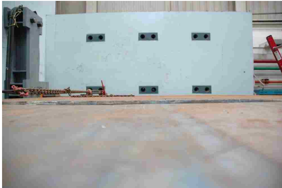
Figure 108 Elevation difference at splice location before tacking
