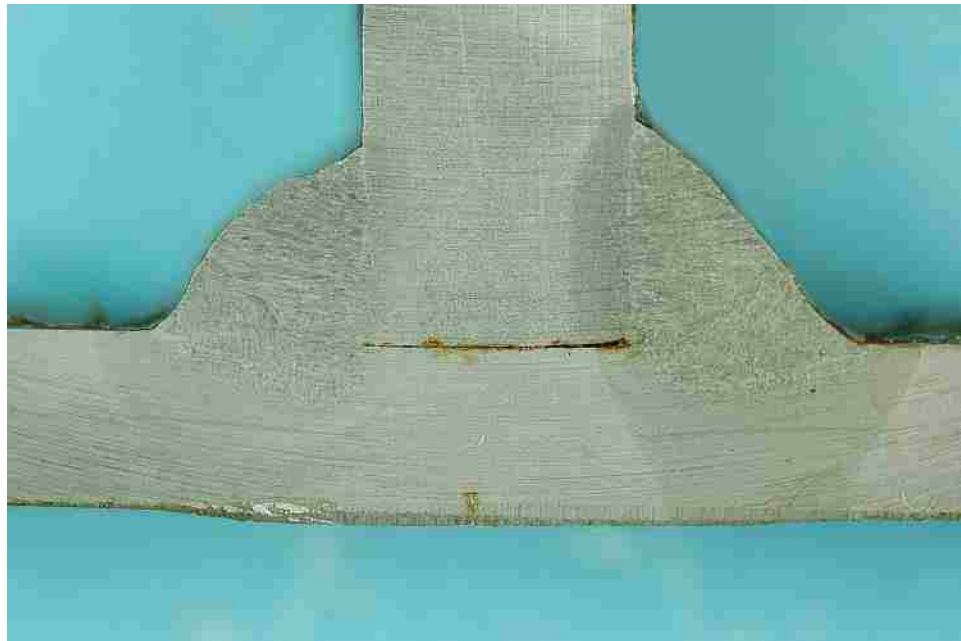
Figure 149 Macro-etched section FS_N_50
