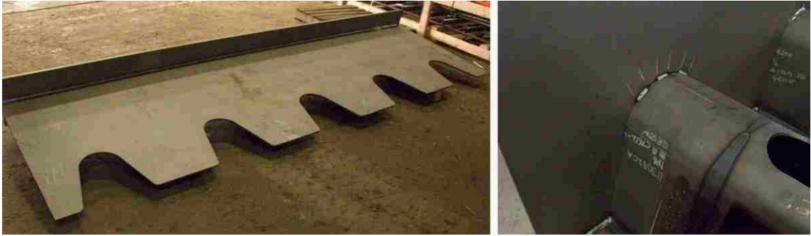
Figure 99 Match-cutting of floor beam for rib-to-floor beam weld
