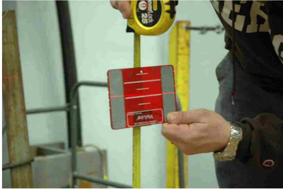
Figure 120 Deck level measurements using laser
