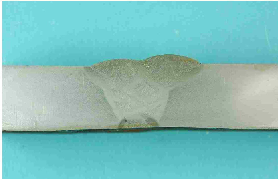
Figure 164 Macro-etched section 3 of CJP deck weld
