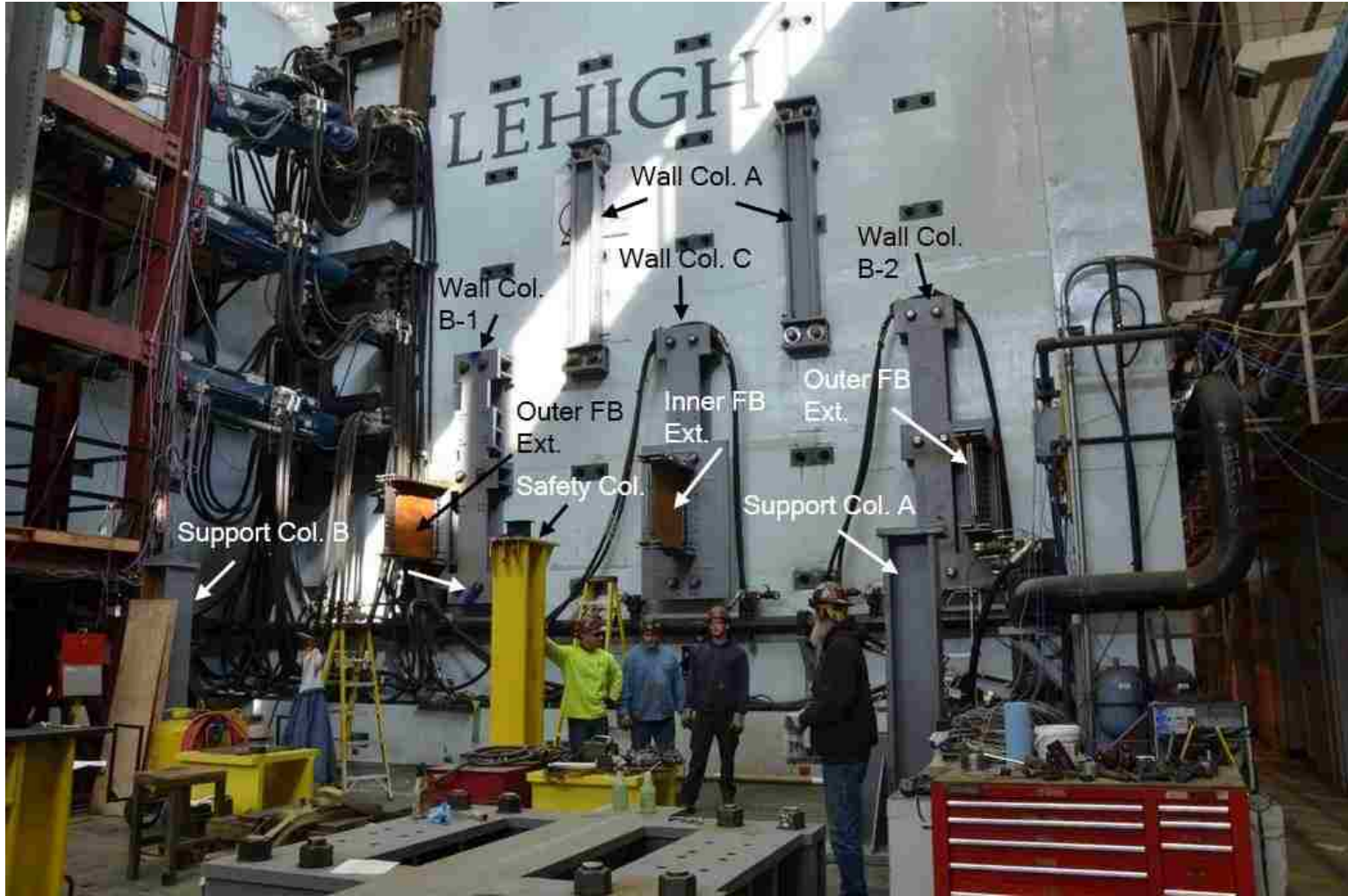
Figure 103 Fixtures for the prototype deck
